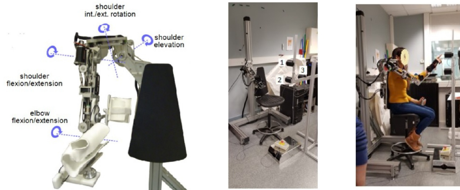
Fig 4. The experimental setup. The ABLExoskeleton imposes a viscous field on the subjects, forcing them to change their kinematic behavior.
