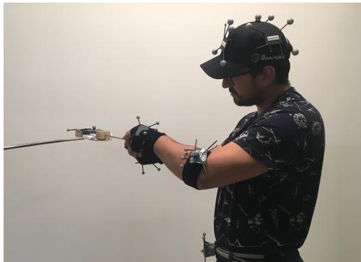
Figure 12: Setup for the data collection. The human performing the task is strapped with multiple markers. Another person is holding a mock object that the user must screw on. This object is also tracked when recording the data. The object is held using a stick to prevent blocking the vision of the object.
