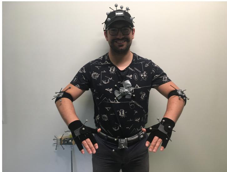
Figure 8: Marker positioning when collecting the data with Optitrack. 8 markers are placed on the body to measure the joints positions and one is placed on the object the human is operating on. Forward Kinematics is then used to extract the joint configuration
