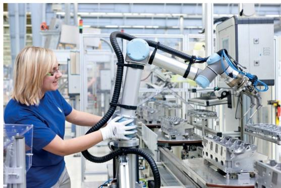
Figure 2: Example of a compliant robot
